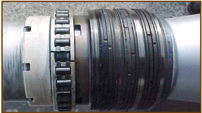
Figure 2. Broken 4½ bearings (like the one shown here) could cause the Prowler aircraft to fail in flight.
