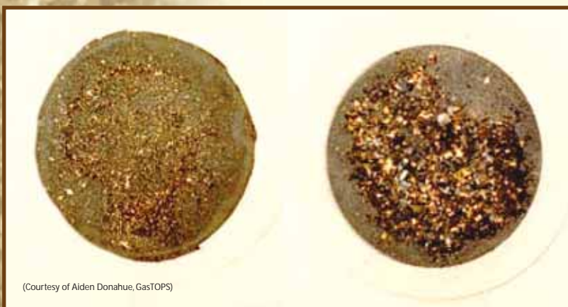
Figure 1. The filter patch on the left shows debris from an operational engine. The patch on the right shows debris from an engine in failure.
